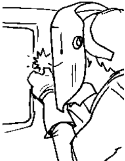
Welding of anchor into the "B" pillar
