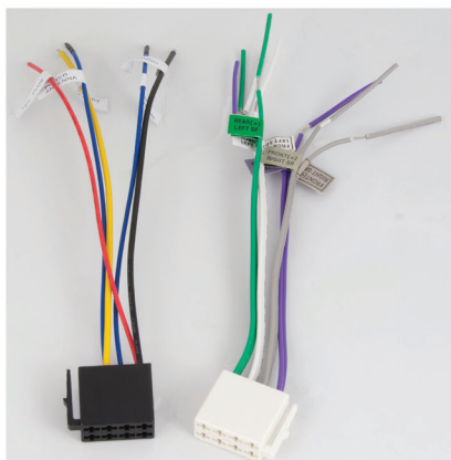
Power/Speaker Wire Harnesses (Plug both into Main Wire Harness)
